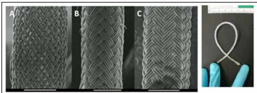
Scanning electron micrographs of three braided conduits using a different number of polymer filaments in the yarn. (A) Single-filament yarn, (B) Three-filament yarn, (C) Triaxial braid with three-filament yarn and longitudinal fibers running along the conduit axis. (Scale bars = 1 mm) (D) Braided conduits bent on wires are extremely flexible and kink-free.
