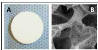
A: Bone regeneration scaffolds made of tyrosine-derived polycarbonates as disks, plates, or strips of a highly porous material that can be cut to size by the surgeon in the operating room, followed by press-fitting the implant into the bone defect.
