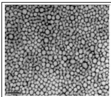
Transmission electron micrograph of tyrosine-derived polymeric nanospheres dispersed in buffer and dried on gold grids. Negative staining with uranyl acetate was applied. Scale bar = 100 nm.
