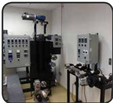
Figure 1. Alex James melt extruder produces biodegradable fibers at up to 100 m/min
