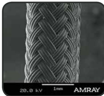
Figure 2. Flexible nerve conduit of braided biodegradable filament
