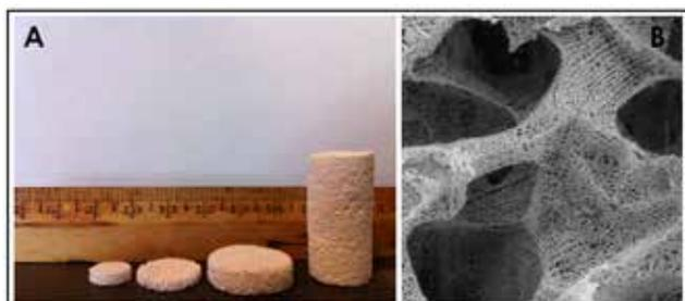
*A) Photograph of tyrosine-derived polycarbonate bone regeneration scaffolds of varying dimensions fabricated by a combination of phase separation, freeze-drying, and salt-leaching. B) Scanning electron micrograph of tyrosine-derived polycarbonate bone regeneration scaffolds showing both macropores (for cell infiltration) and micropores (for diffusion and exchange of nutrients and waste).*
