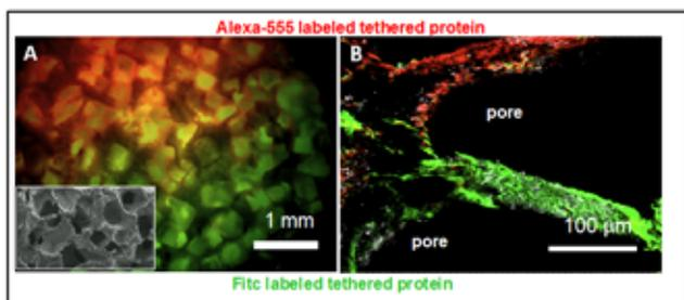
*Spacial tethering of ligands within a single scaffold. (A-B) Confocal images of different fluorescent proteins tethered in a single scaffold forming a distinct interface, inset SEM in A shows pore structure.*
